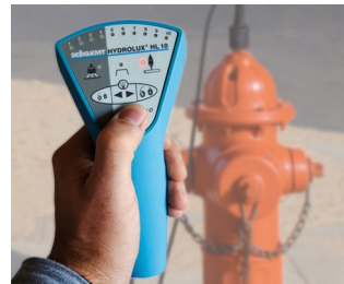
One-handed ground microphone
