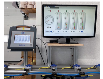
Monitoring system for cleaning nozzles
