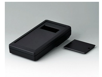
A9074409 DATEC-MOBIL-BOX M, Vers. IV ABS (UL 94 HB) black RAL 9005 195x101x44mm IP 65 opt.
