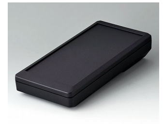
A9075119 DATEC-MOBIL-BOX L, Vers. I ABS (UL 94 HB) black RAL 9005 252x121x50mm IP 65 opt.
