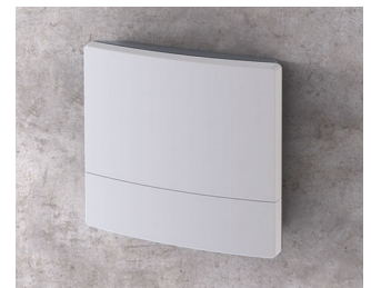
B3218201 NET-BOX 180, Vers. II ASA+PC (UL 94 V-0) light grey RAL 7035 180x180x48,5mm IP 65 opt.
