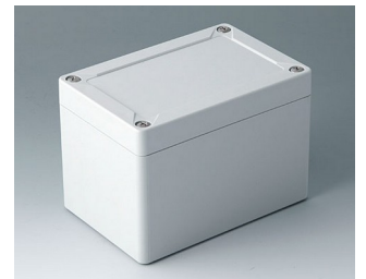
C7012021 IN-BOX ABS (UL 94 HB) light grey RAL 7035 122x82x85mm IP 66, IP 67, IK 07
