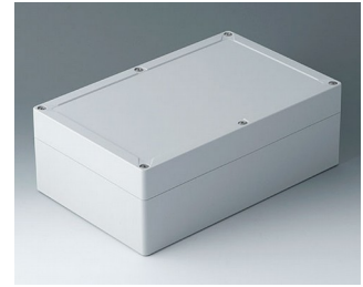
C7025081 IN-BOX ABS (UL 94 HB) light grey RAL 7035 252x162x90mm IP 66, IP 67, IK 07
