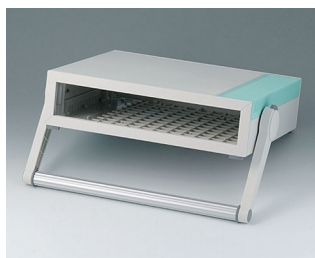
B2210105 MEDITEC D 220, with handle bar ABS (UL 94 HB) off-white RAL 9002 290x260x74mm IP 40
