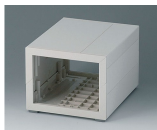
B2213217 MEDITEC E 160, without handle bar ABS (UL 94 HB) off-white RAL 9002 160x200x124mm IP 40
