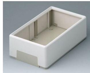
A9540165 FLAT-PACK CASE 210 A ABS (UL 94 HB) off-white RAL 9002 210x125x70mm IP 40
