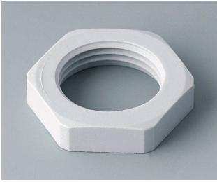
C2320117 Counternut M20x1.5 PA light grey RAL 7035
