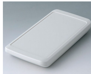
B5403207 SLIM-CASE M, Vers. II ASA+PC (UL 94 V-0) off-white RAL 9002 148x74x19mm IP 65 opt., IP 40
