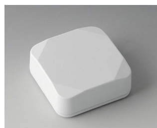
B1804217 MINI-DATA-BOX S50, haute ASA+PC (UL 94 V-0) blanc signalisation RAL 9016 50x50x20mm IP 65 opt., IP 40
