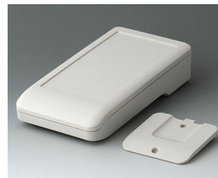
A9006217 DATEC-COMPACT M ASA+PC (UL 94 V-0) gris blanc RAL 9002 172x92x39mm IP 41
