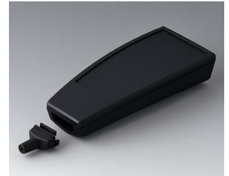
A9067349 SMART-CASE L, Vers. V ABS (UL 94 HB) noir RAL 9005 140x62,7x30,5mm IP 65 opt., IP 40
