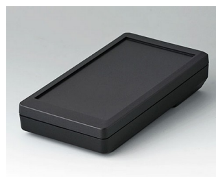
A9073119 DATEC-MOBIL-BOX S, Vers. I ABS (UL 94 HB) noir RAL 9005 152x83x33,5mm IP 65 opt.
