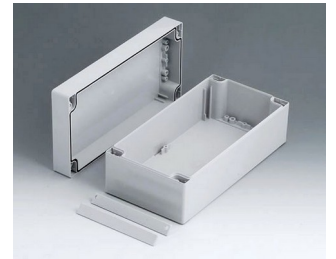
C2112242 ROBUST-BOX 120 LARGE, Vers. II PC (UL 94 HB) gris clair RAL 7035 240x120x90mm IP 66
