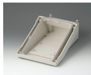
B4016317 DATEC-TERMINAL M, Vers. III ABS (UL 94 HB) gris blanc RAL 9002 168x272x101mm IP 54 opt.
