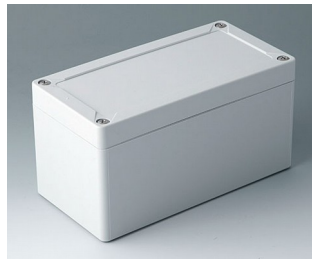
C7016021 IN-BOX ABS (UL 94 HB) gris clair RAL 7035 162x82x85mm IP 66, IP 67, IK 07
