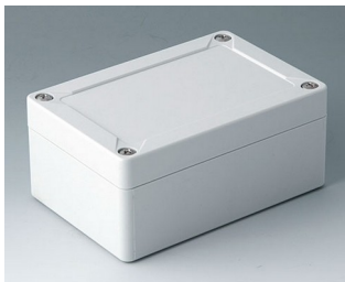
C7012012 IN-BOX PC gris clair RAL 7035 122x82x55mm IP 66, IP 67, IK 08
