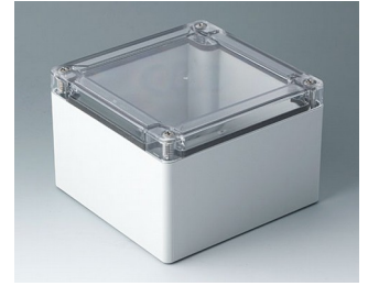
C7013054 IN-BOX ABS/PC (UL 94 HB) gris clair RAL 7035 124x122x85mm IP 66, IP 67, IK 07
