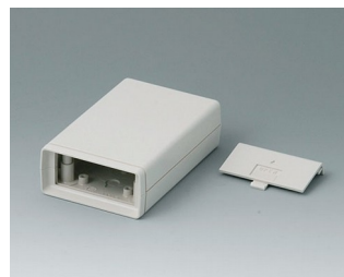
A9406334 BOITIER COQUILLES V 110, Vers. II ABS (UL 94 HB) gris blanc RAL 9002 72x114x33mm
