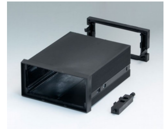
B6032041 BOITIER ENCASTRABLE TYPE A, Vers. I PPO (UL 94 V-0) noir RAL 9005 96x48x109mm
