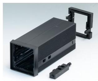
B6012051 BOITIER ENCASTRABLE TYPE A PPO (UL 94 V-0) noir RAL 9005 48x48x114mm
