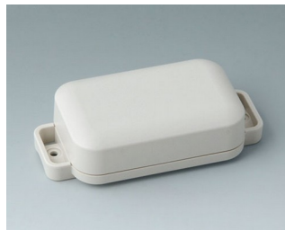
C3204207 EASYTEC 80 ASA+PC (UL 94 V-0) gris blanc RAL 9002 101x50x26mm IP 65 opt., IP 40
