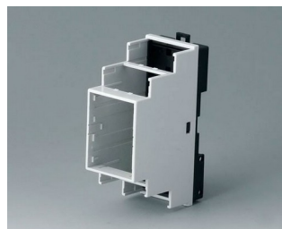
B6501121 RAILTEC B, 2 modules, Vers. VI PC (UL 94 V-0) gris clair RAL 7035 35x90x58mm
