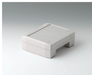
C8011132 SOLID-BOX 115 PC+ABS (UL 94 V-0) gris clair RAL 7035 135x115x50mm IP 66, IP 67, IK 08
