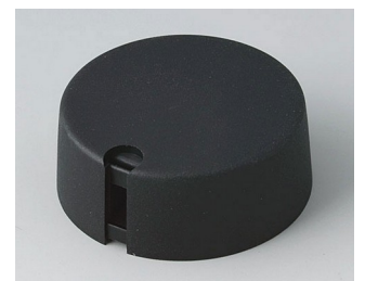
A1040049 TOP-KNOBS 40 PA 6 néro 40x16mm 4mm
