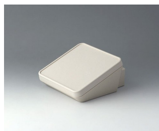
B4414307 PROTEC 140, Vers. III ASA+PC (UL 94 V-0) gris blanc RAL 9002 140x160x76mm IP 65 opt.
