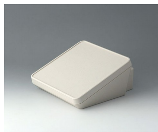
B4418307 PROTEC 180, Vers. III ASA+PC (UL 94 V-0) gris blanc RAL 9002 180x201x92mm IP 65 opt.
