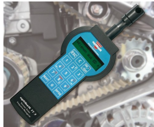
Pretension tester for V-belts and toothed belts
