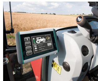
ISOBUS terminal for tractors and self-propelled machines
