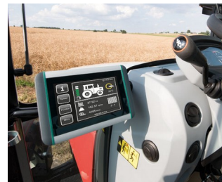
ISOBUS terminal for tractors and self-propelled machines
