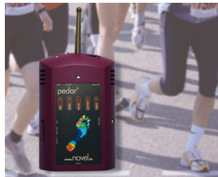
Dynamic pressure measuring between foot and shoe
