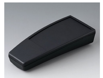
A9068119 SMART-CASE XL, Vers. II ABS (UL 94 HB) black RAL 9005 168x74,4x35,4mm IP 65 opt., IP 40
