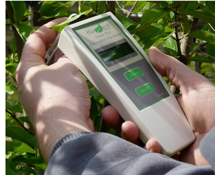
Chlorophyll fluorimeter for plant screening
