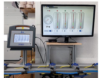
Monitoring system for cleaning nozzles
