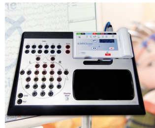
Stationary system for long-term EEG recordings
