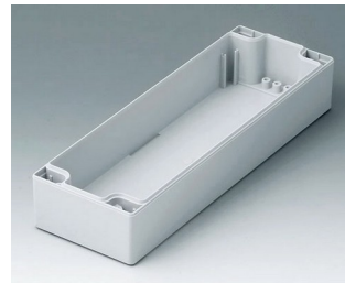
C1082401 Case shell 80, with tongue ABS (UL 94 HB) light grey RAL 7035 240x80x40mm
