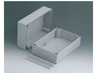
C2416242 ROBUST-BOX WIDTH 160, Vers. II PC (UL 94 HB) light grey RAL 7035 240x160x120mm IP 66
