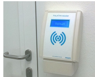
RFID access control readers
