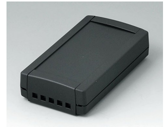
B1055469 TOPTEC 123 F, Vers. II ABS (UL 94 HB) black RAL 9005 123x68x30mm IP 40
