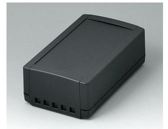
B1070469 TOPTEC 194 H, Vers. II ABS (UL 94 HB) black RAL 9005 194x115x68mm IP 40
