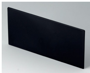
B6143221 Front panel PPO (UL 94 V-0) black RAL 9005 139,3x67,5x2mm
