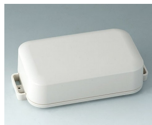
C3208207 EASYTEC 150 ASA+PC (UL 94 V-0) off-white RAL 9002 172x93x46mm IP 65 opt., IP 40
