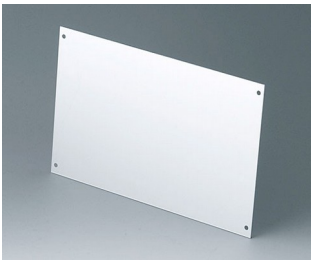
A9180001 Front panel 220 Aluminium matt anodised 205,5x129,4x1,5mm
