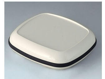
B1608217 BODY-CASE XL, with recess ASA (UL 94 HB) traffic white RAL 9016 62x56x17mm IP 65
