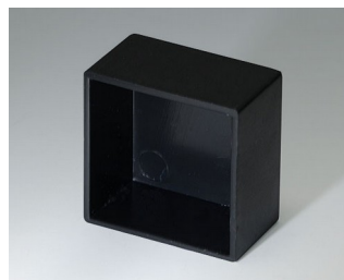
A8021129 POTTING BOXES, Vers. III ABS (UL 94 HB) black RAL 9005 21,2x21,2x12,1mm
