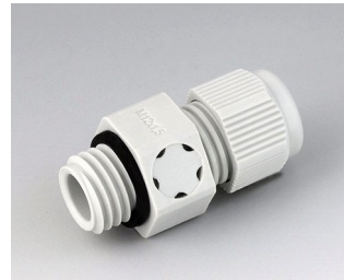
C2312917 Cable gland M12x1.5, pressure compensation PA light grey RAL 7035
