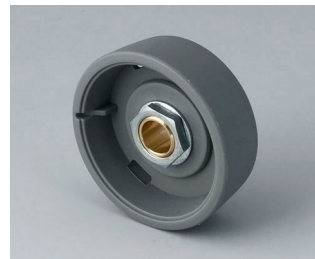
B8033638 STAR-KNOBS 33 PA 6 volcano 33x14mm 1/4"
