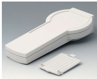
A9076107 DATEC-CONTROL XS, Vers. I ABS (UL 94 HB) off-white RAL 9002 200x94x39,5mm IP 65 opt.
