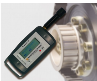
Tension meter for measuring belt pretension
