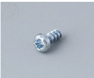
A0304031 Self-tapping screws 2.2 x 5 mm (PZ1)
