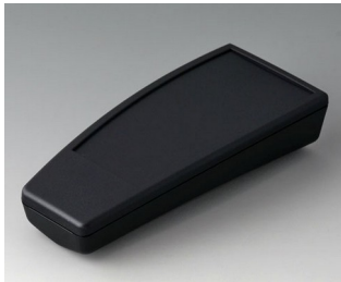
A9067119 SMART-CASE L, Vers. II ABS (UL 94 HB) black RAL 9005 140x62,7x30,5mm IP 65 opt., IP 40
