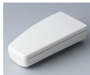
A9066107 SMART-CASE M, Vers. I ABS (UL 94 HB) off-white RAL 9002 96x47x24mm IP 40
