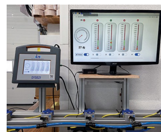
Monitoring system for cleaning nozzles
