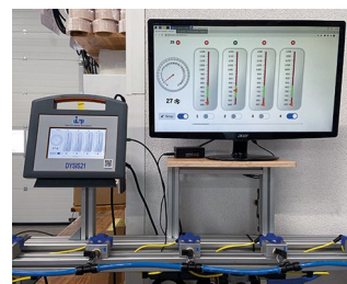
Monitoring system for cleaning nozzles
