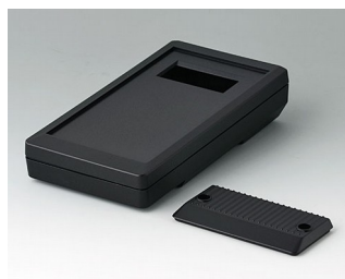
A9073209 DATEC-MOBIL-BOX S, Vers. II ABS (UL 94 HB) black RAL 9005 152x83x33,5mm IP 65 opt.
