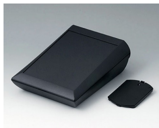
A0615119 COMTEC 150 H, Vers. II ABS (UL 94 HB) black RAL 9005 150x200x71,5mm IP 40
