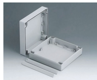
C2016162 ROBUST-BOX WIDTH 160, Vers. II PC (UL 94 HB) light grey RAL 7035 160x160x60mm IP 66
