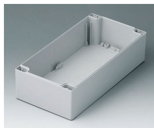
C2122401 Case shell 120, with tongue ABS (UL 94 HB) light grey RAL 7035 240x120x60mm
