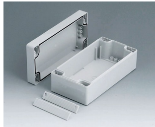
C2008162 ROBUST-BOX WIDTH 80, Vers. II PC (UL 94 HB) light grey RAL 7035 160x80x60mm IP 66
