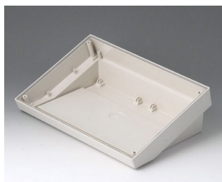
B4026117 DATEC-TERMINAL SL ABS (UL 94 HB) off-white RAL 9002 264x180x86mm IP 54 opt.
