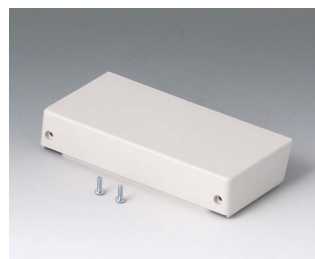
B4016417 Lid M closed, flat ABS (UL 94 HB) off-white RAL 9002 134x62x24mm
