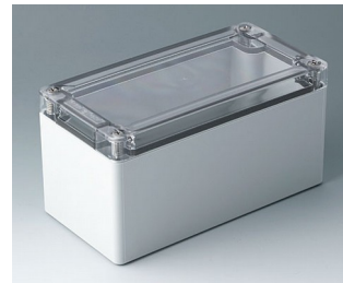
C7016024 IN-BOX ABS/PC (UL 94 HB) light grey RAL 7035 162x82x85mm IP 66, IP 67, IK 07
