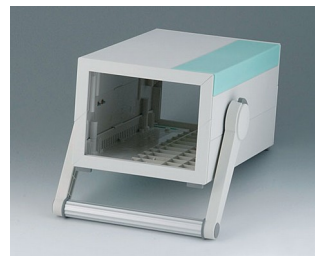
B2212315 MEDITEC E 220, with handle bar ABS (UL 94 HB) off-white RAL 9002 160x260x124mm IP 40
