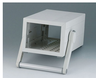
B2212317 MEDITEC E 220, with handle bar ABS (UL 94 HB) off-white RAL 9002 160x260x124mm IP 40
