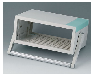
B2211315 MEDITEC D 160, with handle bar ABS (UL 94 HB) off-white RAL 9002 290x200x124mm IP 40
